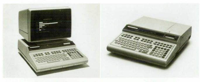
Fig. 1. Model 9835A/B Desktop Computer's large memory capacity and powerful I/O system make it especially well suited for control and data acquisition applications in addition to scientific computation. Model 9835A has a 24-line CRT display. Model 9835B has a single-line display.
