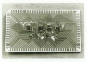
Fig. 5. Existing 9800 Series processor hybrid was modified to accommodate the new address extension chip.
