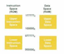
Fig. 2. The processor can directly address two 64K-byte blocks of read-only memory and two 64K-byte blocks of random-access (read/write) memory. Each of these four blocks has a corresponding 16-bit register on the address extension chip. The contents of the register corresponding to a particular block defines which of the 65,536 possible blocks is to be used as that block. Two other AEC registers are for base page read/write and direct memory access.
