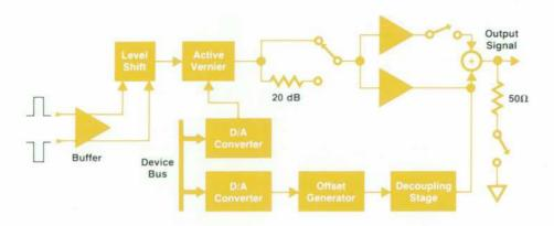
Fig. 15. Organization of the output stage. With the  $50\Omega$  termination switched in, the output stage absorbs reflections from external impedance mismatches. With it switched out, the effective source impedance is 1 k $\Omega$ .
