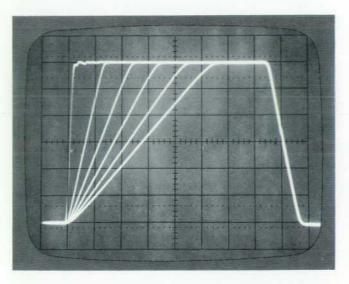
Fig. 14. Minimizing the roll-off effect makes the start of the pulse leading edge virtually independent of the transition time, as shown by this multiexposure photo.
