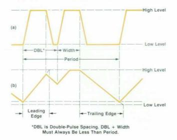
Fig. 5. Errors caused by double pulses running into each other are also allowed by the 8160A, enabling generation of complex waveforms like that shown in (b).
