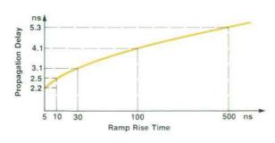
Fig. 8. Propagation delay in an uncompensated VCO Schmitt trigger varies with the rise time of the ramp and therefore varies as the pulse period is changed.
