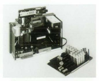
Fig. 16. Power supply with one circuit board removed and another raised in position to disclose details. Although the supply is compact, cooling air is able to flow freely over heatdissipating surfaces.
