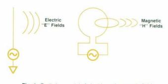
Fig. 1. Radiation model of electric and magnetic fields.
