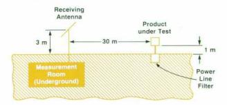
Fig. 3. EMI test range similar to that used by VDE in Offenbach, West Germany. The surface is paved with asphalt and a wire mesh under the asphalt provides a stable reflected wave. required to perform this transformation. The uncertainties of EMI measurements place an additional burden upon the designer in isolating the key variables as well as in setting the design standards.
