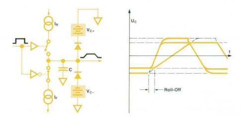
Fig. 12. Conventional slope generator is followed by a limiter stage to remove the step at the start of each transition. Changing the leading edge slope thus affects the start time of the pulse. This is the roll-off effect.
